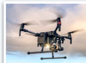
The Matrice 210 V2 carries our FLIR XT2 sensor, and the Z30 offers 180x zoom for asset inspections at a safe distance
